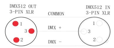
Termination reduces signal errors and to avoid signal transmission problems and interference. It is always advisable to connect a DMX terminal. (Resistance 120ohm 1/4W) between pin2(DMX-) and pin3(DMX+) of the last fixture.
